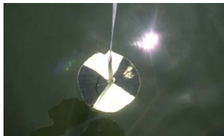
Figure 1 Secchi Disc being Lowered into BCR
